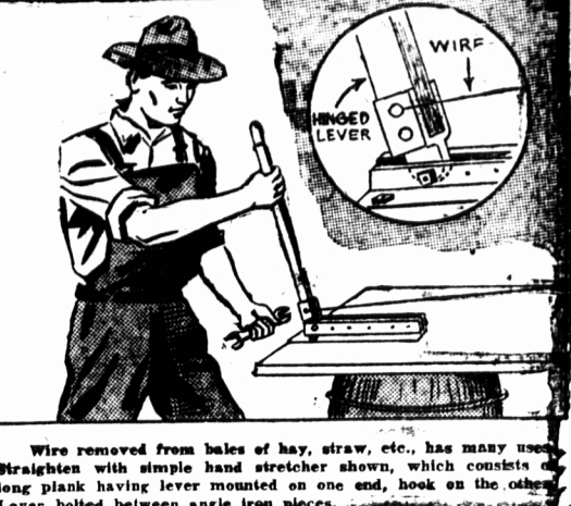
Wire removed from bales of hay, straw, etc., has many uses. Straighten with simple hand stretcher shown, which consists of long plank having lever mounted on one end, hook on the other. Lever bolted between angle iron pieces.
