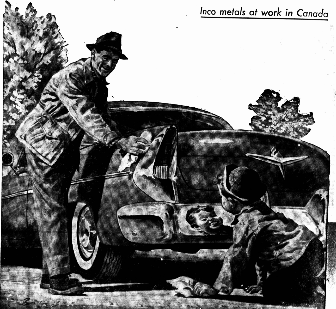
We ordinarily speak of automobile bumpers, grilles, hubcaps and bright metal trim as being "chrome-plated". Actually, these parts are plated with both nickel and chromium—a heavy coating of nickel covered with a thin layer of chromium. All the nickel used for plating auto parts and other products of Canadian industry is Inco nickel—mined, milled, smelted and refined in Canada.
