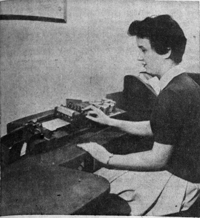
MISS FAYE PROUDE is seen verifying the information punched on IBA cards. This machine is used to eliminate any mistakes made in punching the cards.
