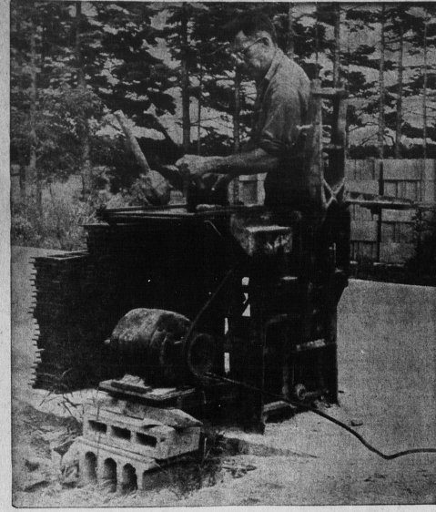
STEPHEN BURKE OPERATES CEMENT BLOCK MACHINE
