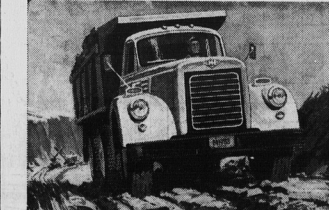
V-Series—G.V.W. ratings range from 25,000 to 50,000 lbs., with a choice of models and three bonus power V-8 engines from 206 to 256 horsepower.
