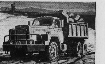
F-210-D Series—A choice of Cummins or Rolls Royce diesel power with G.V.W. ratings up to 48,000 lbs. Also, the F-230-D model at 60,000 lbs. G.V.W. rating.
