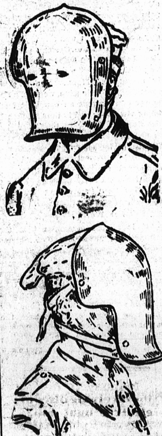
This steel helmet, worn by German sharpshooters on sniping duty, is formed of metal bent so that it will deflect bullets. It is out away on the right side to allow sighting the rifle.
